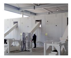
As for extraction units, this is particularly true for units for large milling machines, bar milling machines, or plate saws, as well as centralized extraction units for several different machines. In these cases, automatic handling of swarf and filings offer a better solution, as it optimizes machining processes. However, even without upstream extraction systems due to circumstances and space conditions, an automatic swarf handling unit can be beneficial.
